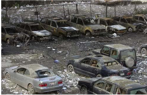
Figure yy. The cars parked in the back suffered extensive damage. The car on the left and on the far right look like they have had their engines eaten. The cars in the foreground experienced less damage, but many windows are missing, however partial and whole windows also remain.
