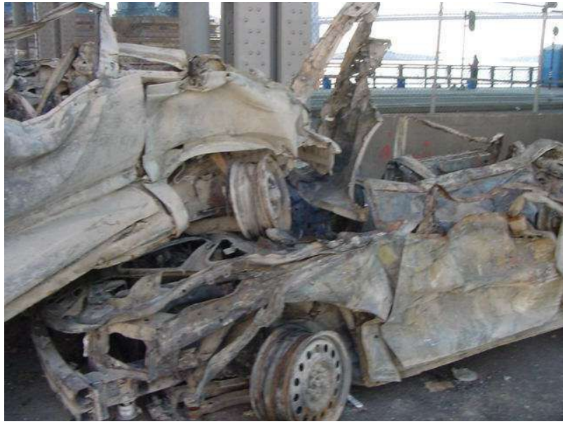
Figure 66(b). Wheels appear to have steel-belts from the tires still on them.
