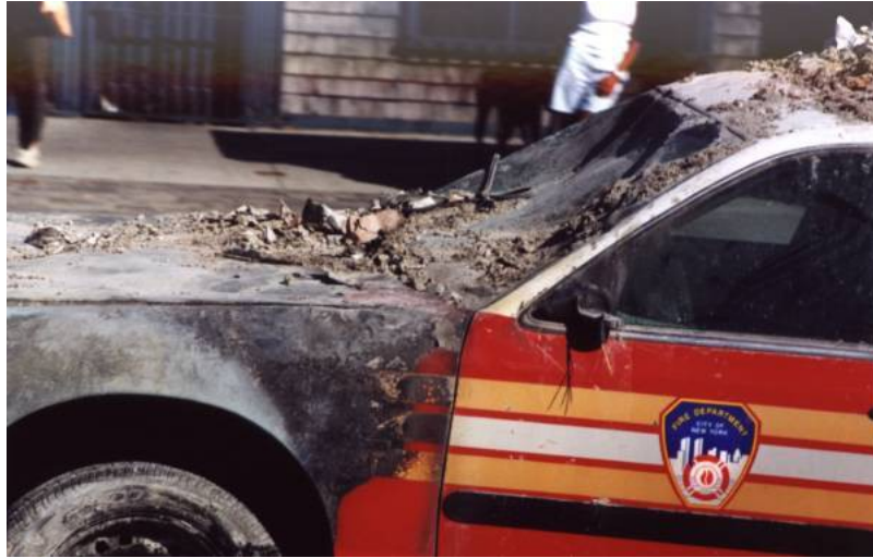
Figure 66(j). The front end of this FDNY car is toasted and mildly deformed, while the door appears undamaged and the window glass is intact. The debris on this car suggests it was near the WTC.
