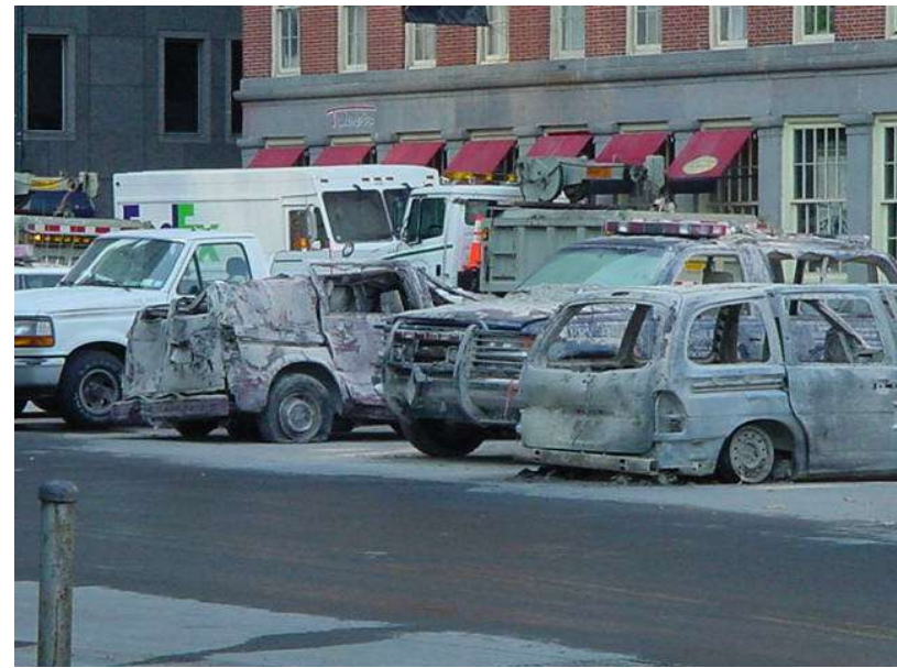
Figure 72. The car with the flat tire appears to have "wilted" from heat, from the top down, leaving a peeling appearance on the back end. The SUV on its right is missing all its window glass except for the windshield. The vehicle on the far right has no trace of tires, no door handles, no tail lights, and no windows. Why?
