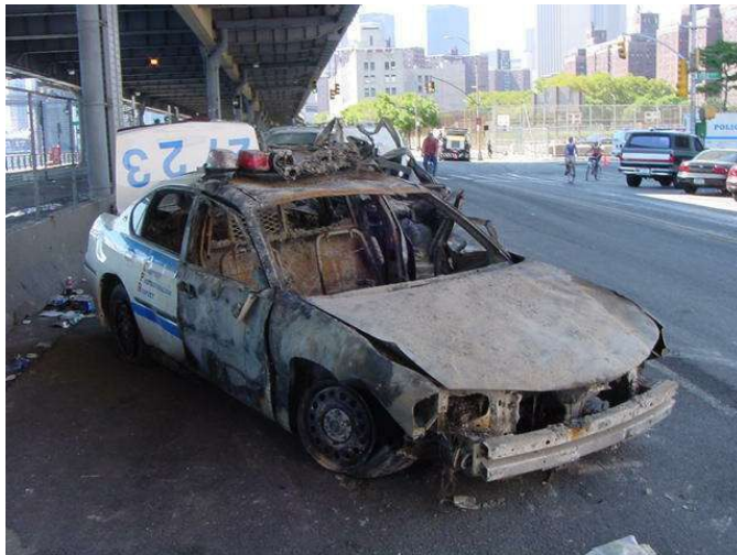
Figure 68. Front half of a car burned with a shiny, unburned rear end.
