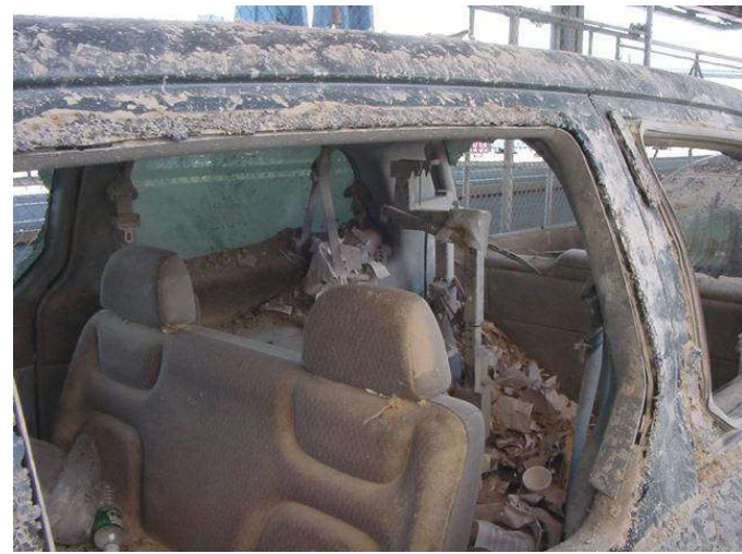
Figure 67. Blistered car on FDR Drive with unburned upholstery and unburned plastic window molding.
