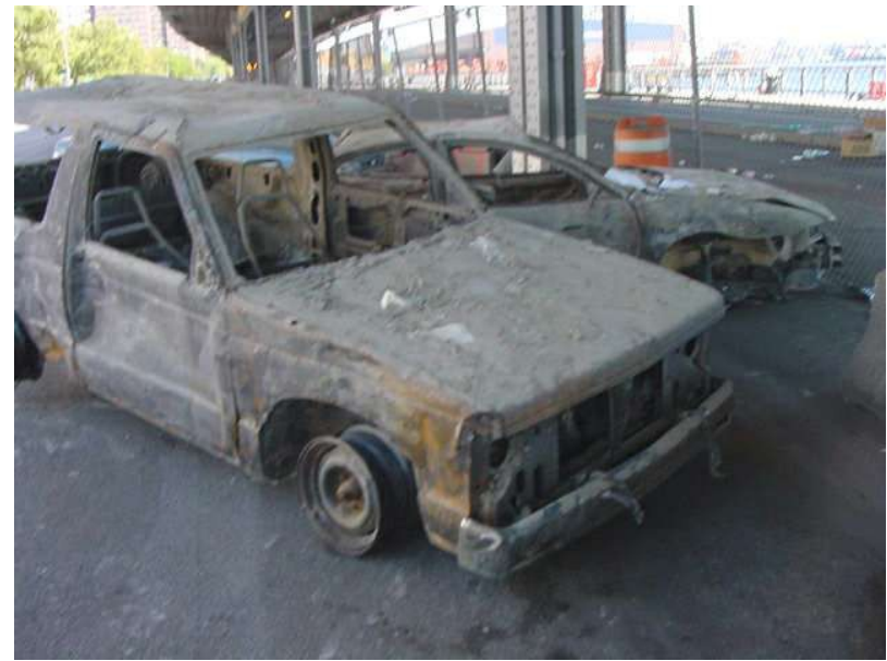
Figure 66(f). While the bodies of these toasted vehicles still exist, they've been incinerated. All of the softer materials inside and out have disappeared.
