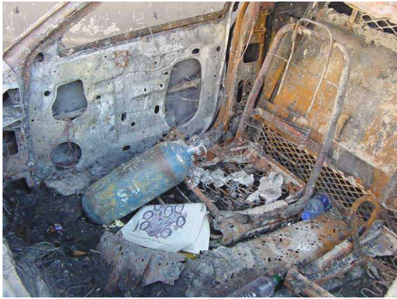
Figure 66(k). This Toasted Interior was consumed except for the fire extinguisher.
