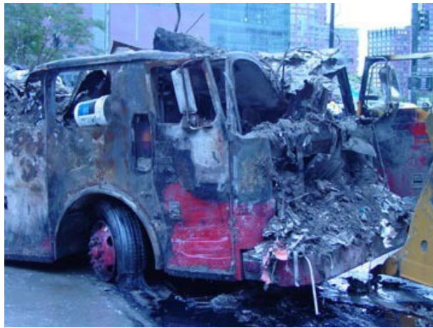
Figure firetruck. A badly damaged firetruck. Where did its engine go? The bottom of the tire has turned to goo below a distinct horizontal line in the tire.
