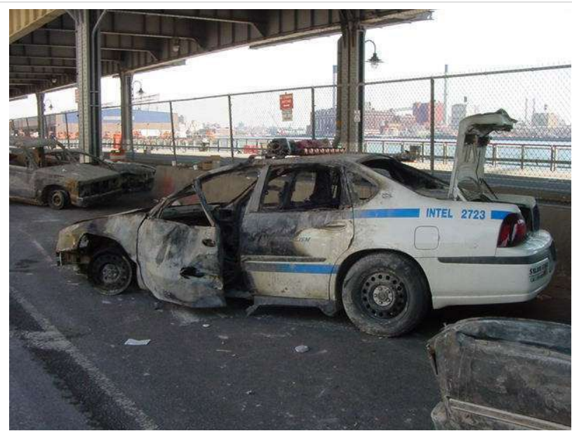
Figure 66(n). There is extensive damage to the front of car 2723, including no door handle on the driver's door. There is an unusual, unburned circular area on the rear door.
