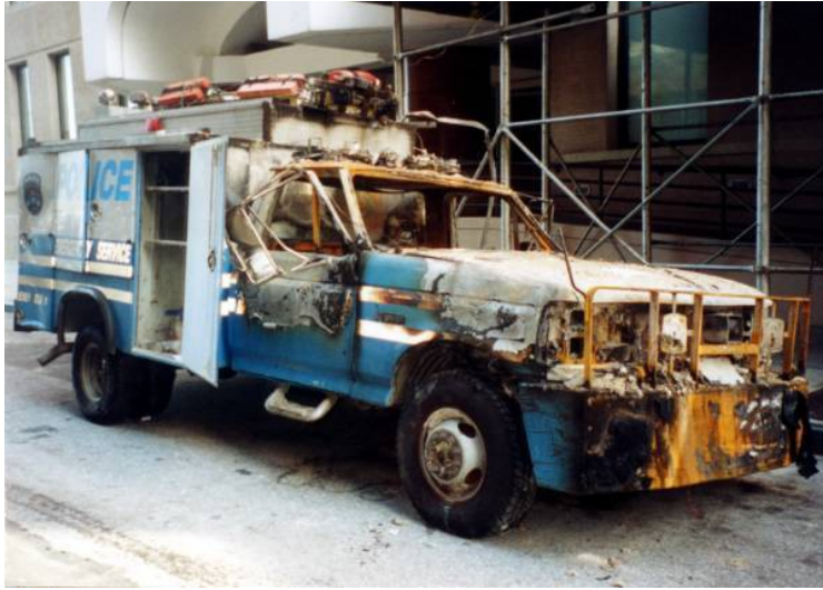
Figure 73. The peeling on the side door appears to be delaminated. Sheet metal is not laminated, so why would it do this?
