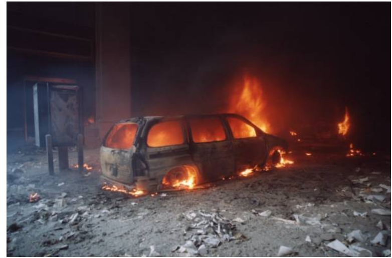
Figure 66(i). A minivan is consumed by flames. The fire rages inside the vehicle, contained by the remaining windows. The fire appears more intense at the front where the engine is.
